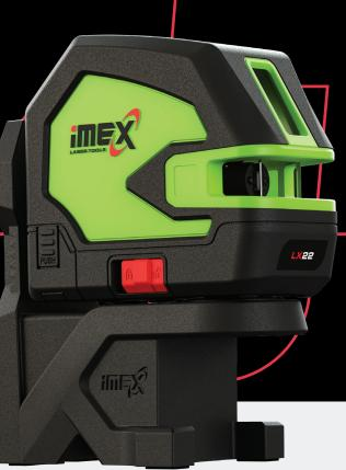
The small, line laser from iMEX with a pulsating beam for outdoor use with optional detector, emitting a strong horizontal and vertical line for all set-out work. With a plumb spot and 360° turn table is a tool for all professional trades. Has a quick release heavy duty magnetic bracket.
