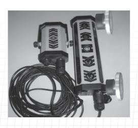
The MR360 is supplied with remote display, which can be connected to the receiver by the special cable. By installing the remote display inside the cabin this will enable you to view the indicating arrows directly rather than always focusing your eyes on the machine's cutting edge, which makes it possible to locate the receiver higher than the cab to prevent laser beaming blocking and to ensure 360 degree reception.
