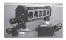
Charge the inside rechargeable battery by the special 240 V charger, the charging time is 6 hours.
